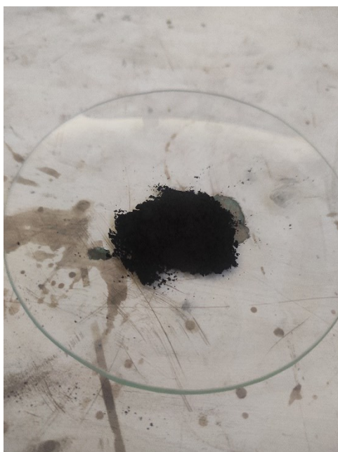
FIGURE 1. NMC 442 cathode result via carbonate co-precipitation method
