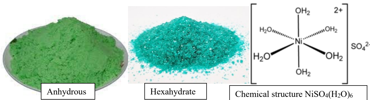
FIGURE 1. Nickel Sulphate in form of anhydrous and hexahydrate, and its chemical structure
