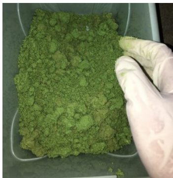
FIGURE 1. MHP produced by PT. Smelter Nickel Indonesia at Balaraja, Banten Province.
