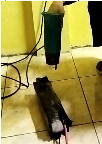
FIGURE 6. Wrap the module with PVC wrap heat shrink.
