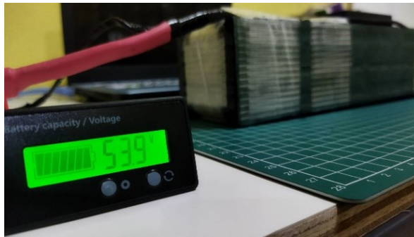
FIGURE 8. Voltage value of battery module after charged 100%.
