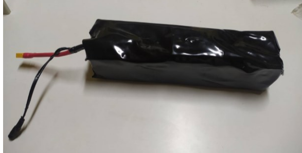
FIGURE 7. The battery module after totally wrapped.
